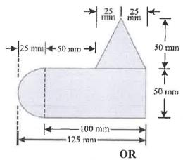
Determine the centroid of the area shown in the figure below with CO3 L4 6 respect to the axis shown.
